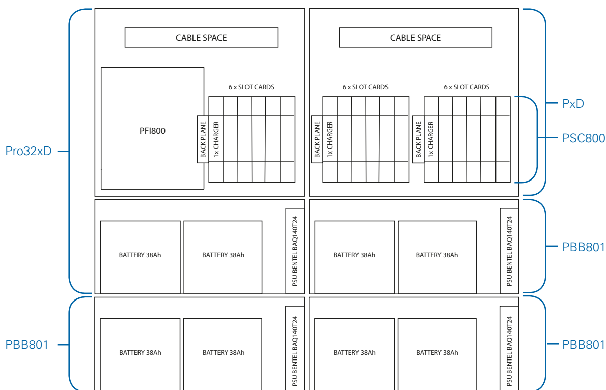
Modular panel consisting of 1 x Pro32xD, 1 x PxD, 1 additional PSC800 and 3 additional x PBB801
