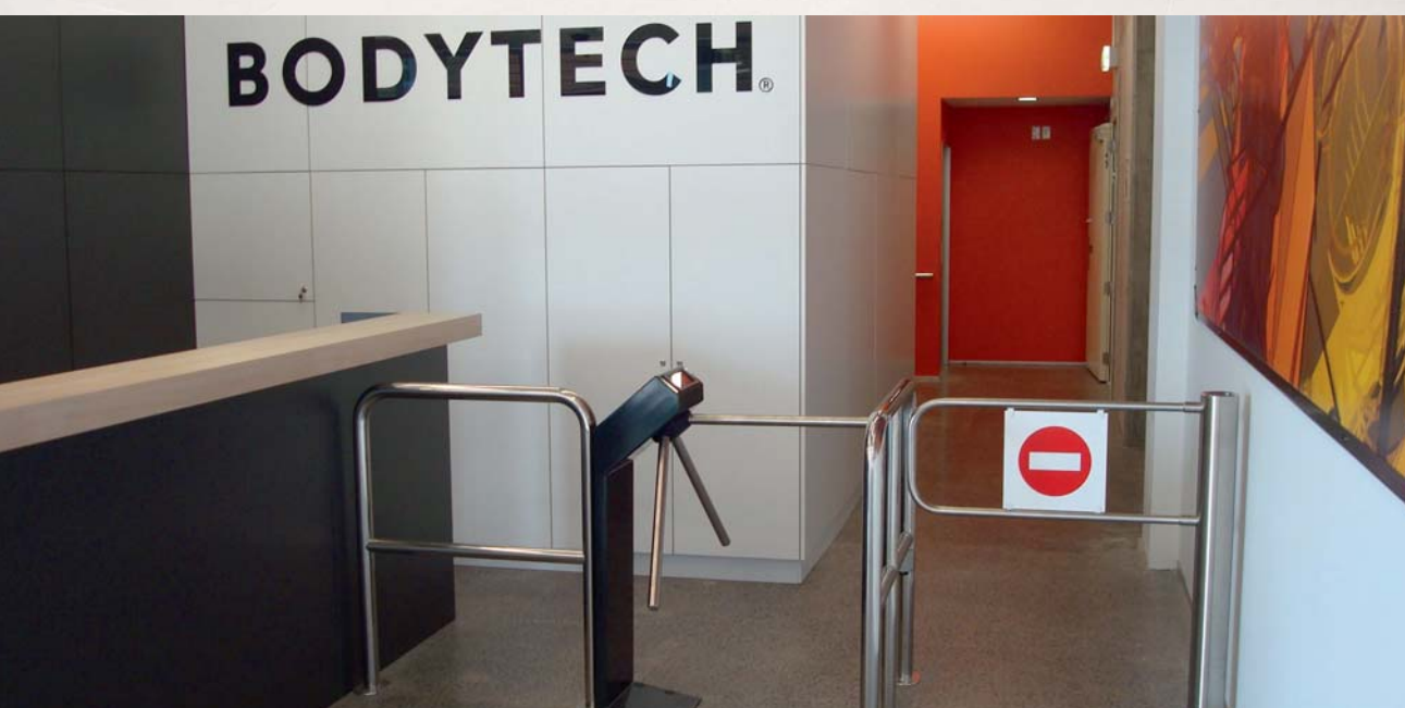
WMD-05S motorized wicket gate with TTR-04.1E tripod turnstile, Bodytech fitness centre, New Zealand
